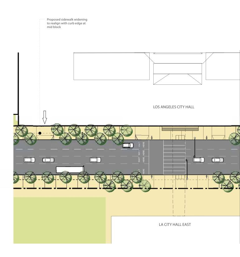
Proposed staggered street tree pattern - spacing 22' o.c. (not more than 25' o.c.)
