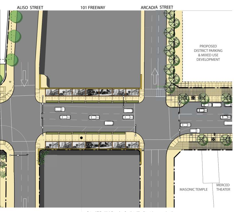
Extend El Pueblo's Boundary South to Aliso Street, incorporating the Freeway Bridges. Develop Gateway "Galerias" that include planters, shade structure, sound barriers, lighting, and canvas art on Both Sidewalks of Main Street and Spring Street bridges while developing preliminary planning for three potential lids over the 101 freeway
