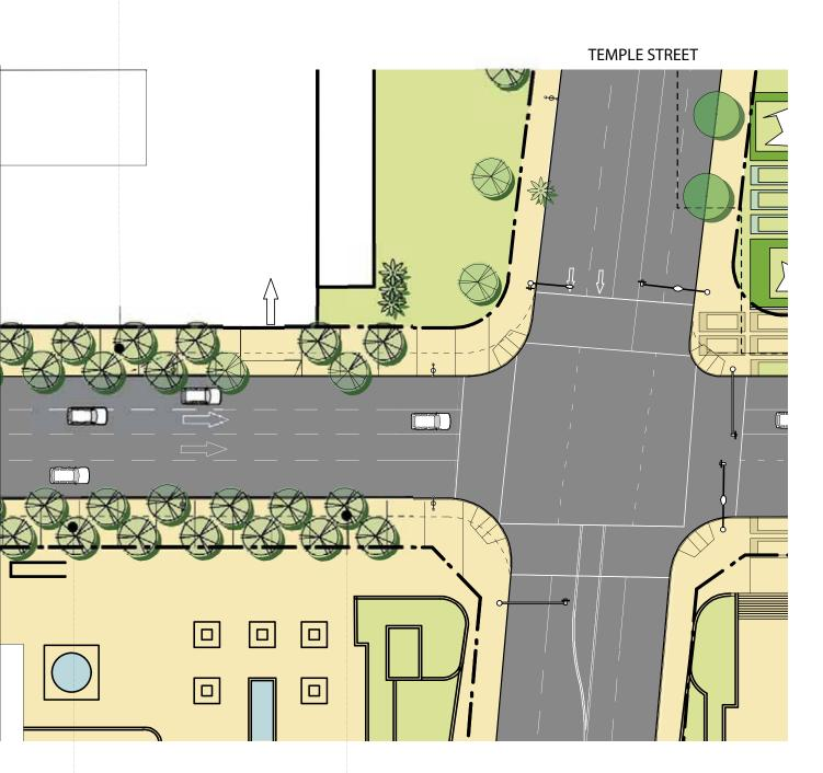
Tree wells - minimum 24" box trees shall be planted in 5' wide X 8' or larger tree wells set back 2' from face of curb planted with low-growing groundcover or perenials, except within 4 feet of the trunk or covered with 3" thick layer of stabilized decomposed granite or covered by a tree grate per Guidelines
